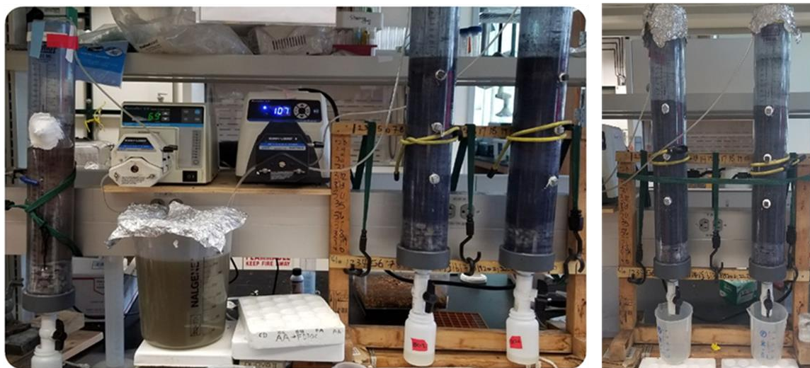
Figure 2: Three columns were set for the selection of biochar (Left) and two columns were set for performance evaluation of biochar amendment rates (Right).
