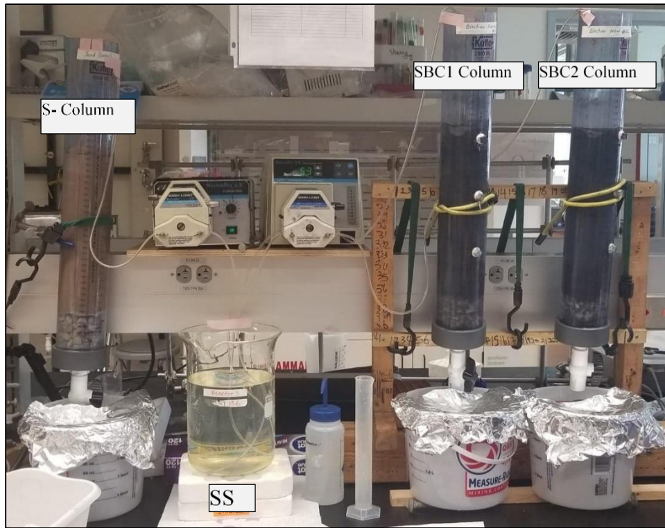
Figure 15: Experimental Setup for stormwater runoff experiment for three columns.
