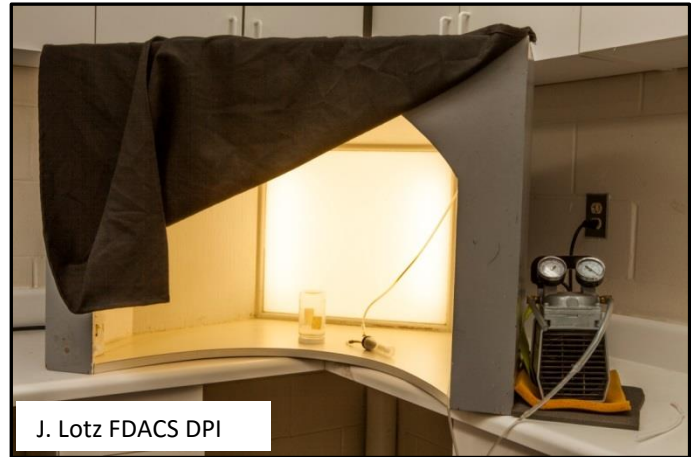
Figure 4: Lighted sorting hood with aspirator and collection vial.
