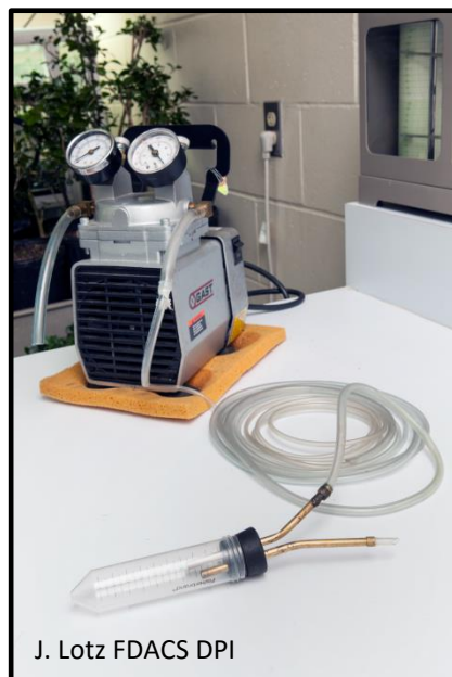
Figure 3: Aspirator assembly with attached collection vial.
