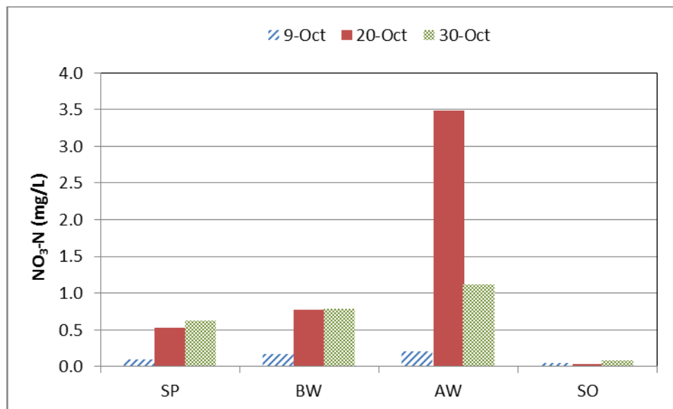
Figure 5. Mean nitrate nitrogen ( \text{NO}_3\text{-N} ) concentrations (mg/L) for three samples collected Oct. 9, 20, and 30, 2014 from spillway runoff (SP), before proposed wall location (BW), after proposed wall location (AW), and shower water (SO). Samples were collected after a wagon of containers passed under the shower at watering station.
