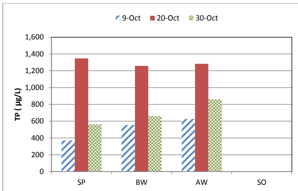
Figure 7. Mean total phosphorus (TP) concentrations (µg/L) for three samples collected Oct. 9, 20, and 30, 2014 from spillway runoff (SP), before proposed wall location (BW), after proposed wall location (AW), and shower water (SO). Samples were collected after a wagon of containers passed under the shower at watering station.
