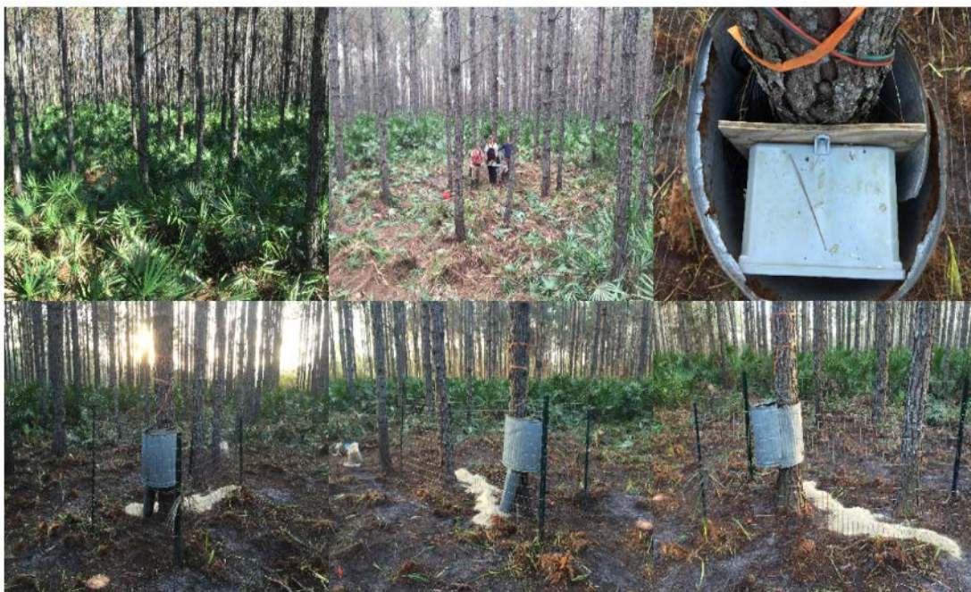
Figure 5: Fire preparation at Green Swamp. Top row, from left: dense saw palmetto understory before burn; field crew clearing vegetation from the area around the datalogger; datalogger protection mechanism; protected data logger. Bottom row: completed site protection with protected data logger and sand barrier to protect exposed cables.
