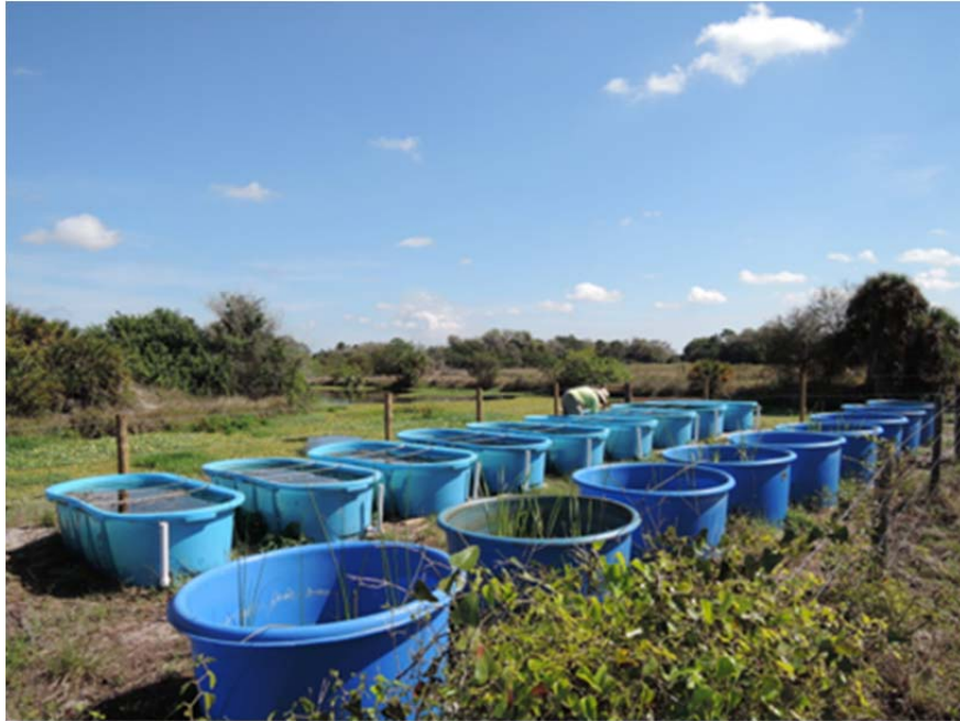
Figure 21. Mesocosm facility at the Hilliard project site, adjacent to the inflow canal. Pictured are the EAV (foreground) and SAV mesocosms.
