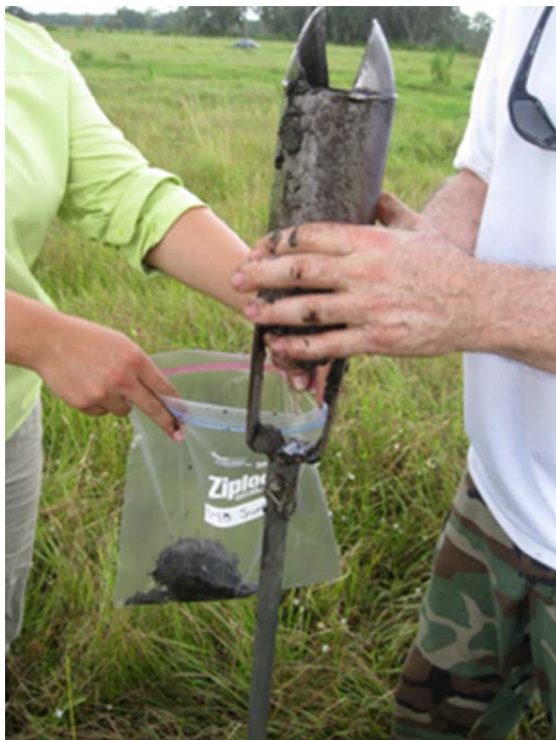
Figure 25. Soil collection using a bucket auger. Soil samples were collected at 40 sites within the FAVT project boundaries for initial chemical characterization.
