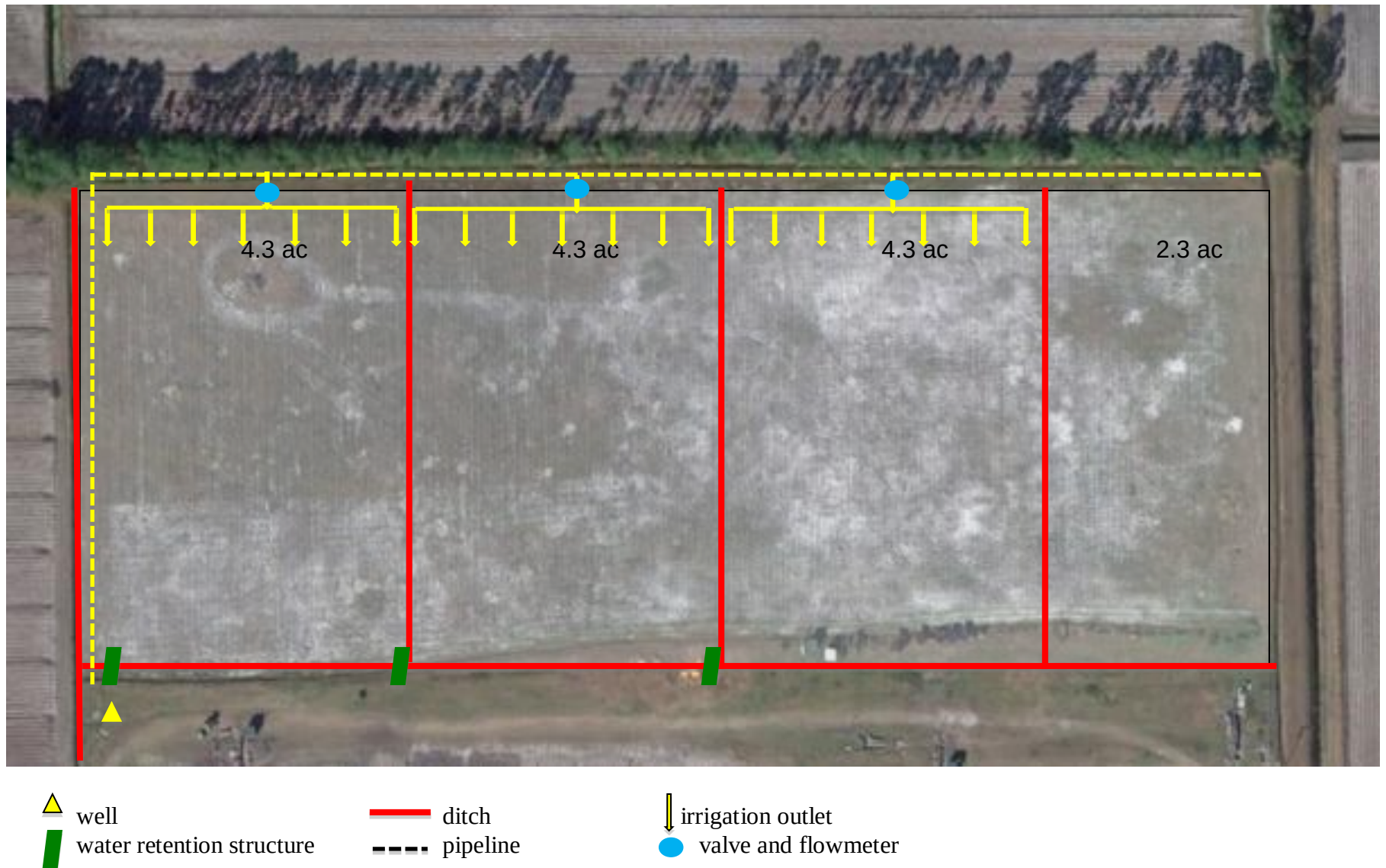
Figure 1. Layout of irrigation and drainage structures on an aerial photograph of the 15.2 acre area at the Experimental Station of Florida Partnership for Water, Agriculture & Community Sustainability at Hastings. (obs. figure not in scale).
