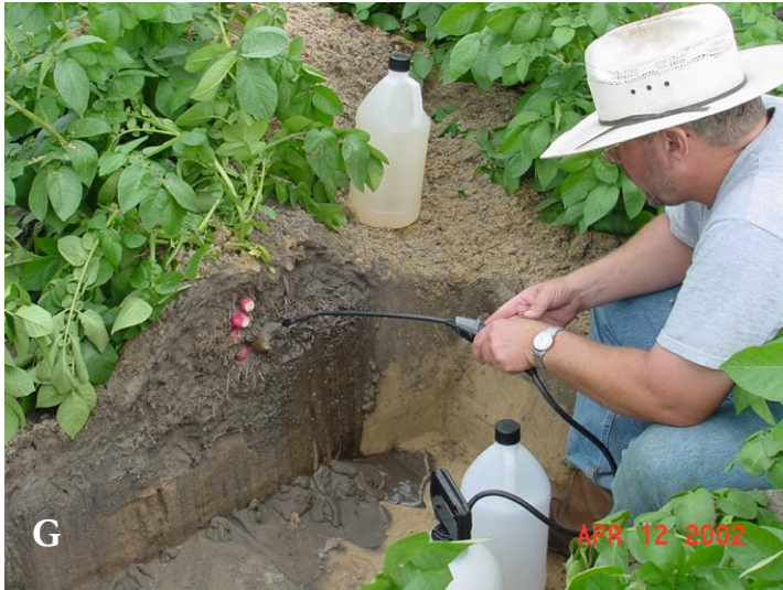
Figure 3 (continued). Use of dye tracer to mimic N and water movement in a potato bed.
