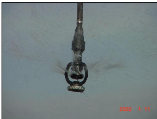
Figure 2. New nozzles placed on the center pivot irrigation system to improve water application characteristics.
