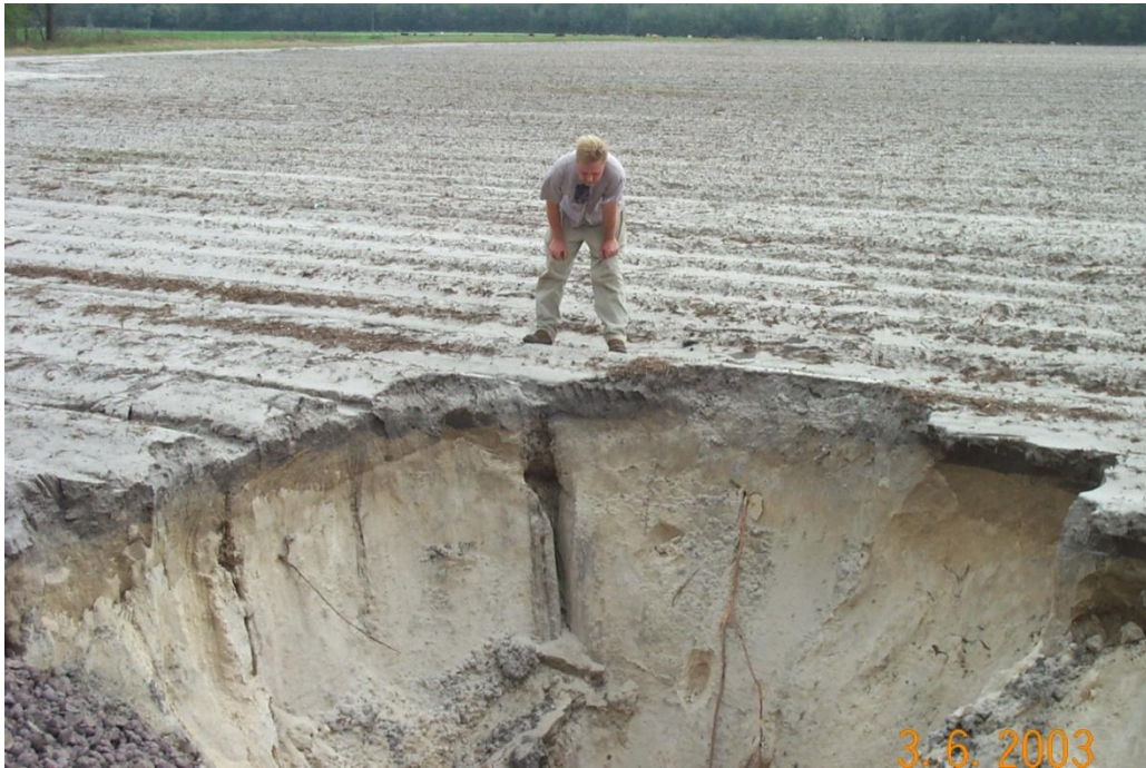
Figure 10. An example of a sinkhole that opened in the demonstration field during the course of the project. Also note the open channels that were exposed by the sinkhole.
