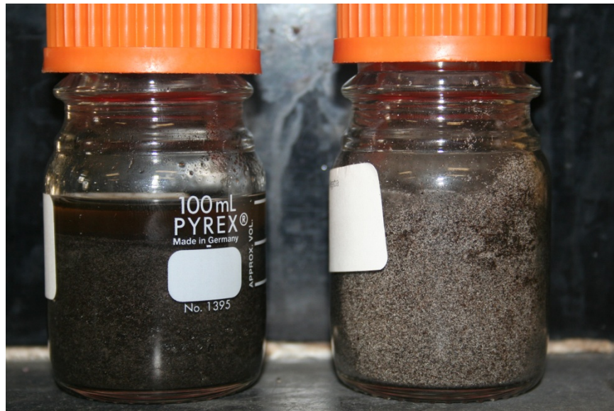
Plate 2. Mesocosm study set up. A) Samples held at 30 °C in the dark. Containers were randomly rotated within incubator and maintained at correct water content by the addition of distilled deionized water on a weekly basis. B) Detail of deep marsh soil with Bahia leaf litter amendment held under flooded (left) and field capacity (right) conditions.
