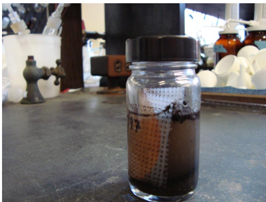
Figure 31 Secured iron strip in bottle with soil and deionized water
