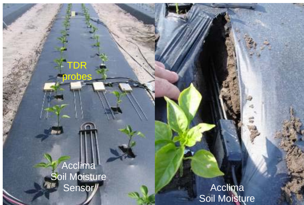
Figure 6. TDR probes and Acclima soil moisture sensor installation (4/20/07).
